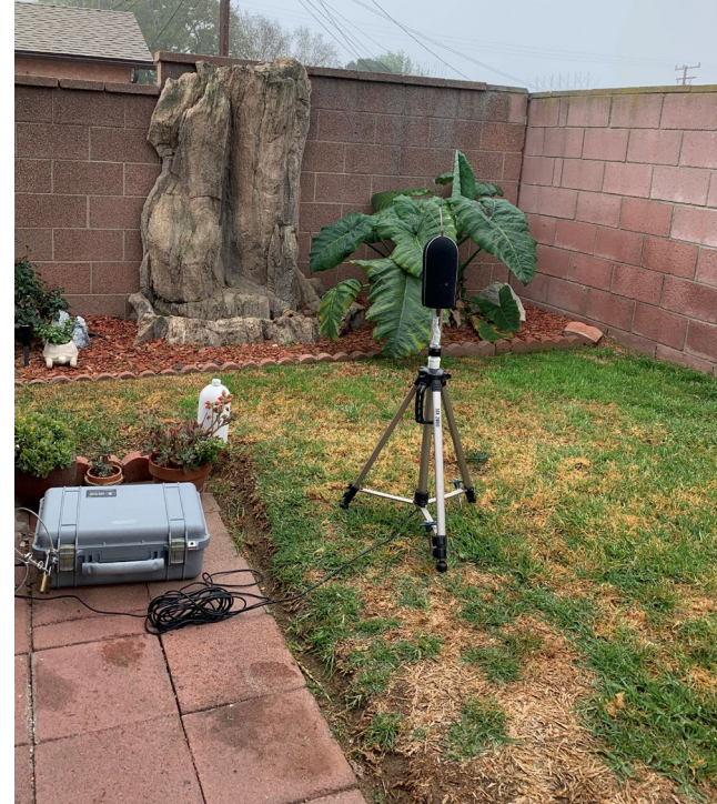
Equipment setup consists of a briefcase-sized box and a camera tripod with a microphone.
